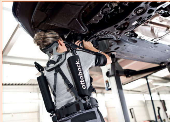
Fig. 6: Paexo neck and shoulder in an assembly line © Ottobock
