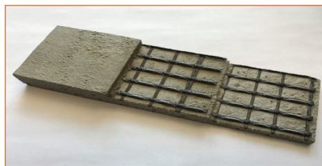
Fig. 3: Textile-reinforced concrete © (ITA Aachen)
